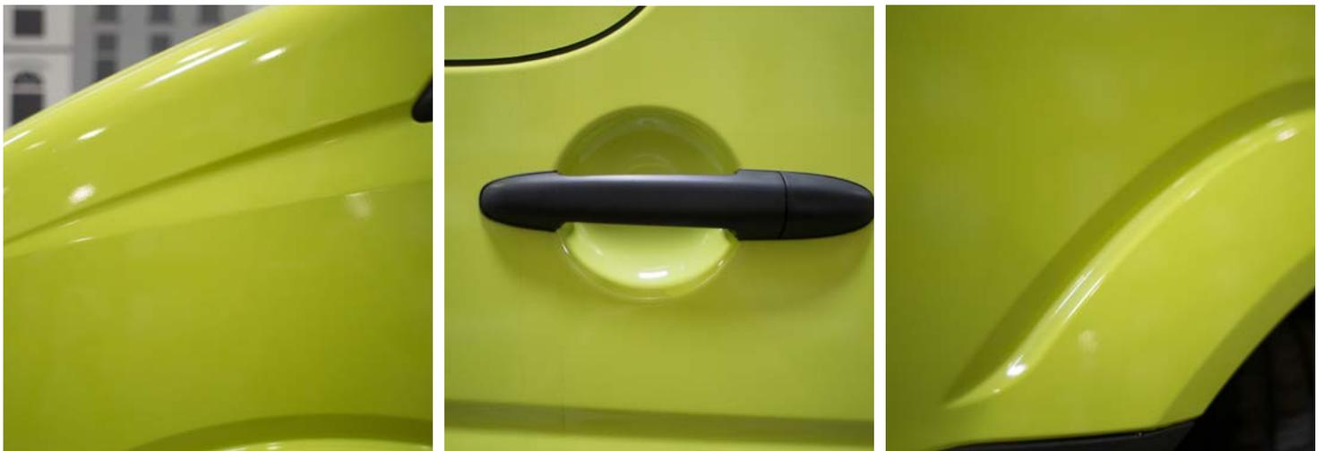
Wrapped in SLX™ Cast Wrap with Series 3270 Overlaminate by OC Wraps
